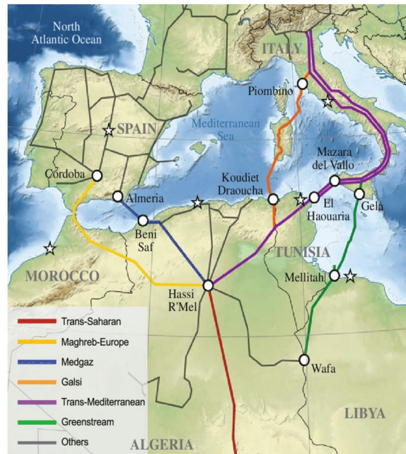
Figure 5: Existing natural gas pipelines from North Africa to Europe.
