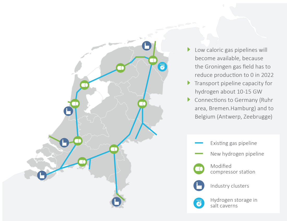
Figure 5 Hydrogen Backbone the Netherlands – Existing natural gas transport pipeline will be converted into a hydrogen transport pipeline that connects hydrogen supply to hydrogen storage and demand in industrial clusters (Gasunie, 2019)
