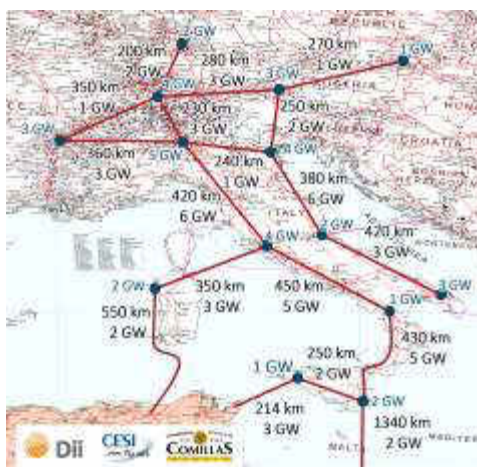
Figure 9 Grid reinforcement Central corridor Option II
