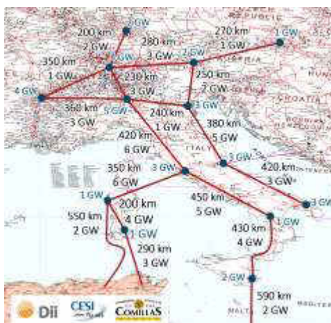
Figure 10 Grid reinforcement Central corridor Option III
