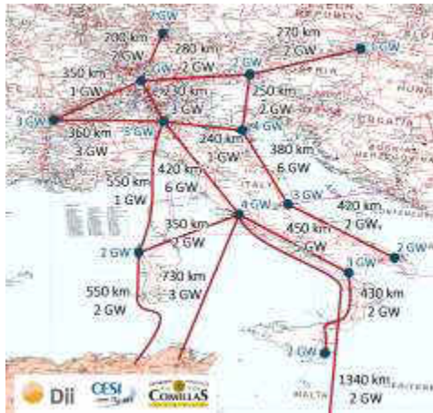
Figure 8 Grid reinforcement Central corridor Option I
